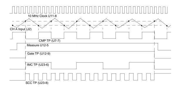
Figure 3-1. Frequency Measurement Timing Diagram
