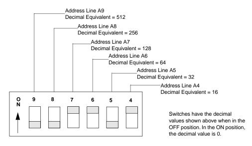
Figure 2-1. The Base Address Switch (Default Base Address of 320h Shown)
