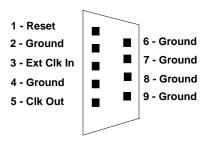
Figure 2-3. Pin Assignments of the 9-Pin "D" Connector
